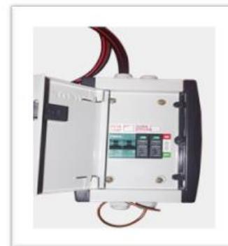
**DC Prewired Box:** Comes with 1 x 63A DP DC MCB, 1 x 2P DC SPD and earthing terminal. Box has cables connected on outside where you have terminals to connect your solar input and solar output.
