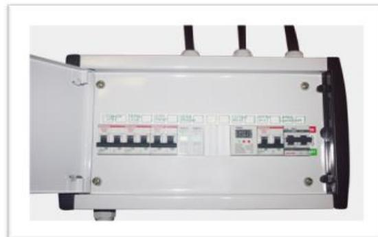
**AC Prewired Box:** Comes with 3 x 25A DP AC MCB, 1 x 10A DP AC MCB, 1 x Voltage Regulator, 1 x 2P AC SPD, 1 x 40A Changeover and earthing terminal. Box has cables connected on outside where you have terminals to connect your grid input and output cables.
