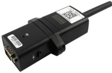
Wi-Fi module enables wireless communication between Flin Inverters and our monitoring platform. Once you connect the module with inverter using communication cable and install the app for it, you can view the operations of the inverter as well as change any settings or parameters as required through the mobile phone.
