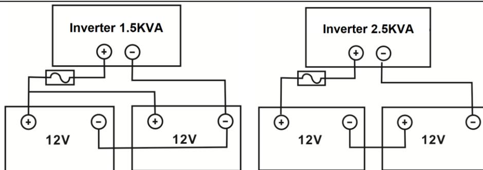
5. Insert the battery wires flatly into battery connectors of inverter and make sure the bolts are tightened with torque of 2 Nm in clockwise direction. Make sure polarity at both the battery and the inverter/charge is correctly connected and conductors are tightly screwed into the battery terminals.
