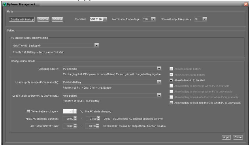
**PV energy supply priority setting:** 1<sup>st</sup> Battery, 2<sup>nd</sup> Load and 3<sup>rd</sup> Grid.
