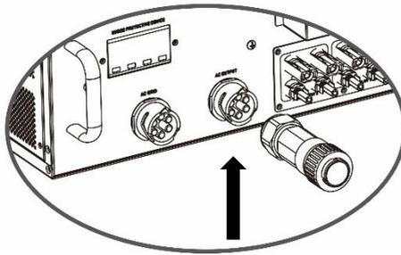
**CAUTION:** It's only allowed to connect load to "AC Output Connector". Do NOT connect the utility to "AC Output Connector".
