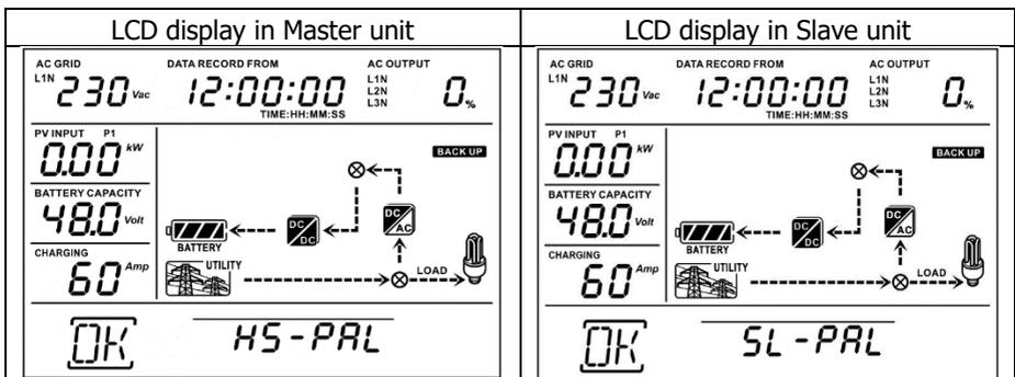
Step 5: If there is no more fault alarm, the parallel system is completely installed.
