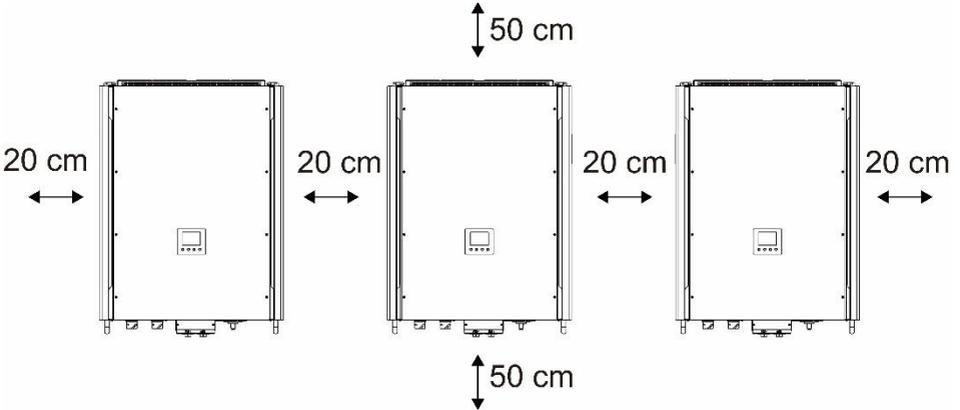
**NOTE:** For proper air circulation to dissipate heat, it's necessary to allow a clearance of approx. 20 cm to the side and approx. 50 cm above and below the unit. Be sure to install each unit in the same level.
