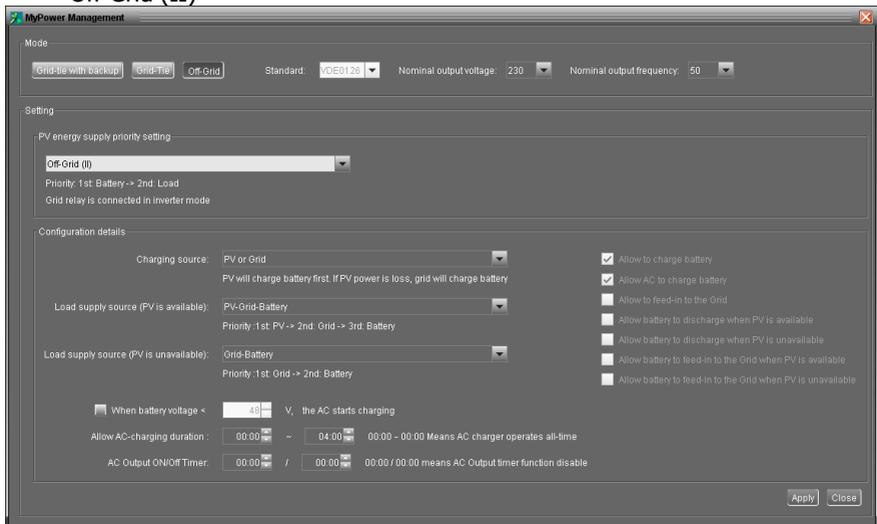
**PV energy supply priority setting: 1<sup>st</sup> Battery, 2<sup>nd</sup> Load**
