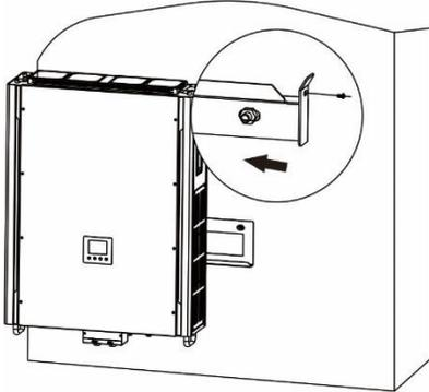
4. Check if the inverter is firmly secured.
