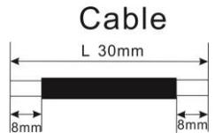
Insert striped cable into female terminal and crimp female terminal as shown below charts.
