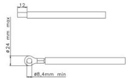
Step 3: Remove battery cover and follow battery polarity guide printed near the battery terminal! Place the external battery cable ring terminal over the battery terminal.
