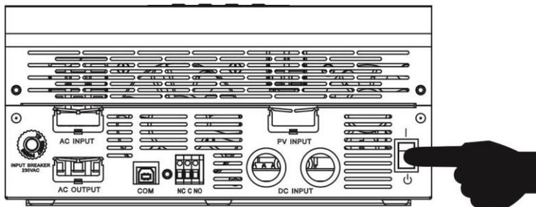
Once the unit has been properly installed and the batteries are connected well, simply press On/Off switch (located on the button of the case) to turn on the unit.
