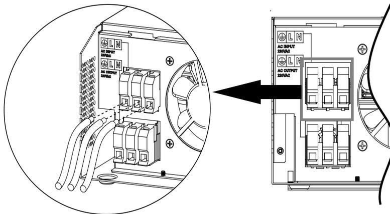
**WARNING:** Be sure that AC power source is disconnected before attempting to hardwire it to the unit.
